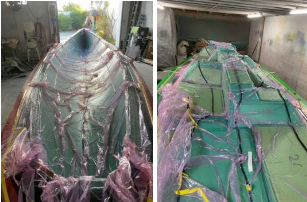
DKG Hull and Internal being Infused separately before being fitted together
