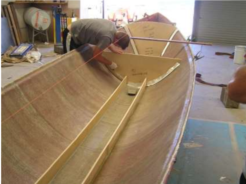
South Coast Surfboat being Laid up in the Single Skin method
